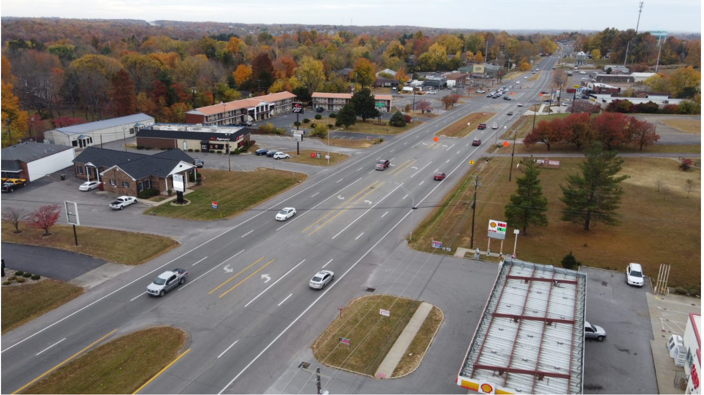
Figure 5: Uncontrolled Parallel Left Turn Lanes
