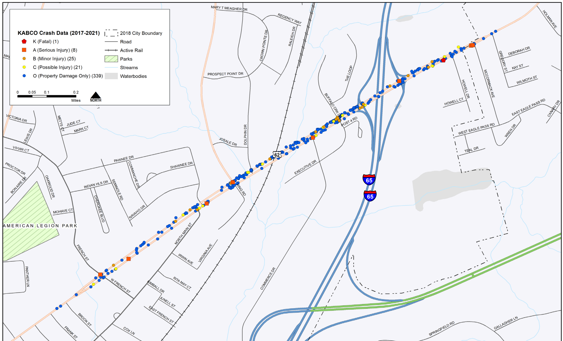
Figure 13: US 62 Crash Severity by Location (2017-2021)
